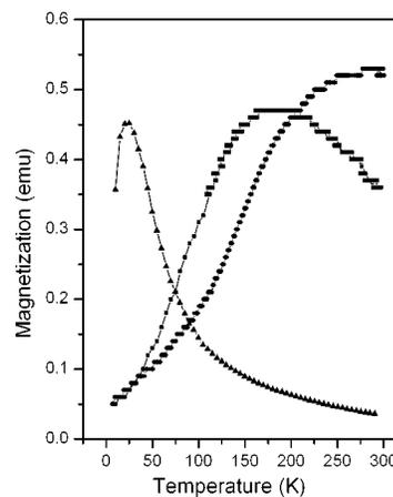
**Figure 10.** Magnetization versus temperature for 4 (triangles), 13 (squares), and 16 nm (circles)  $\gamma$ -Fe<sub>2</sub>O<sub>3</sub> nanocrystallites with zero-field cooling at the applied magnetic field of 100 Oe. The magnetic studies were conducted with a Quantum Design MPMS SQUID magnetometer.
