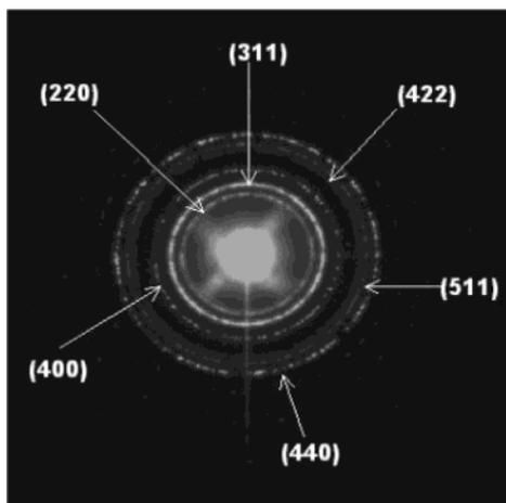
**Figure 3.** Electron diffraction pattern of 11 nm  $\gamma$ -Fe<sub>2</sub>O<sub>3</sub> nanocrystallites.
