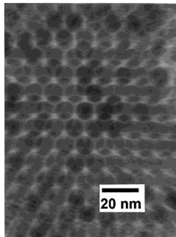
**Figure 5.** TEM image of a three-dimensional superlattice of 11 nm  $\gamma$ -Fe<sub>2</sub>O<sub>3</sub> nanocrystallites.
