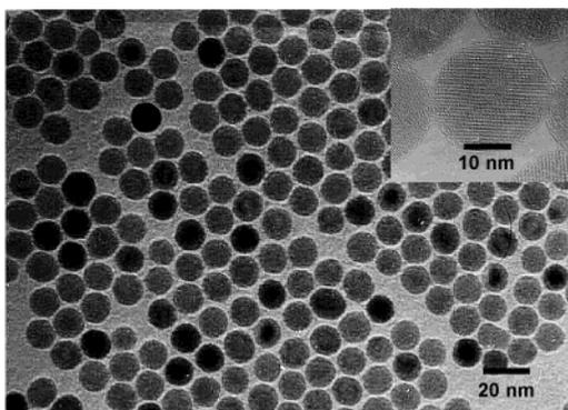
**Figure 9.** Low-resolution and high-resolution TEM image of a single nanocrystallite (inset) of 13 nm  $\gamma$ -Fe<sub>2</sub>O<sub>3</sub> nanocrystallites.
