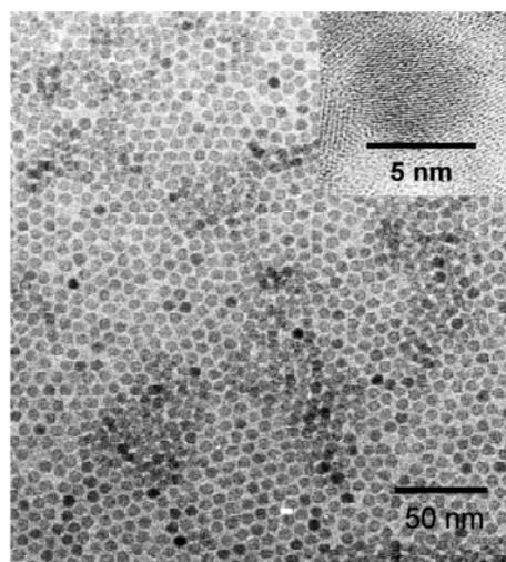
**Figure 6.** Low-resolution TEM image and high-resolution TEM image of a single nanocrystallite (inset) of 7 nm  $\gamma$ -Fe<sub>2</sub>O<sub>3</sub> nanocrystallites.
