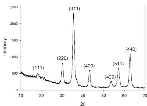
**Figure 4.** X-ray diffraction pattern of 11 nm  $\gamma$ -Fe<sub>2</sub>O<sub>3</sub> nanocrystallites.
