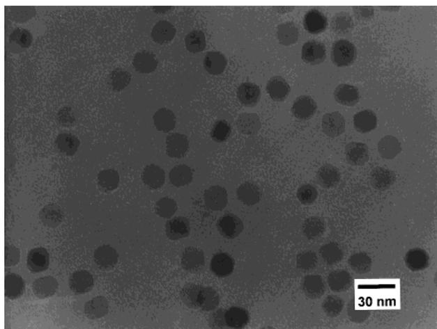
**Figure 8.** TEM image of 16 nm  $\gamma$ -Fe<sub>2</sub>O<sub>3</sub> nanocrystallites.
