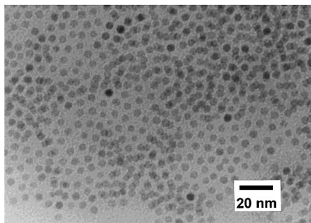
**Figure 7.** TEM image of 4 nm  $\gamma$ -Fe<sub>2</sub>O<sub>3</sub> nanocrystallites.
