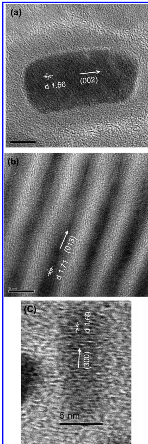
**Figure 7.** (a) HRTEM image of 8 nm × 16 nm sized MnP nanorod. (b) HRTEM image of 7 nm × 600 nm sized FeP nanorod. (c) HRTEM image of 4 nm × 9 nm sized Ni<sub>2</sub>P nanorod.
