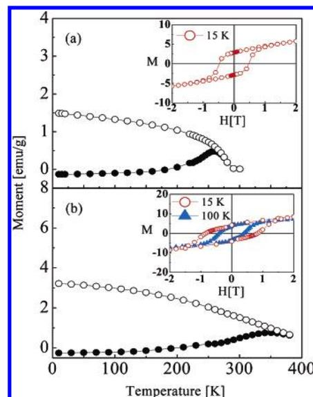
**Figure 9.** The temperature dependence of magnetization for (a) 11 nm  $\times$  25 nm MnP and (b) 11 nm  $\times$  450 nm FeP sample measured with an applied field of 100 Oe after zero-field cooling (filled circles) and field cooling (open circles). The inset displays the field dependence of the magnetization of (a) MnP at 15 K and (b) FeP at 15 and 100 K.
