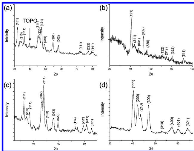
**Figure 6.** X-ray diffraction patterns of (a) MnP nanorods, (b) Co<sub>2</sub>P nanorods, (c) FeP nanowires, and (d) Ni<sub>2</sub>P nanorods.
