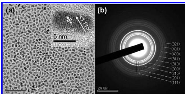
**Figure 5.** (a) Normal TEM image and (b) electron diffraction patterns of Ni<sub>2</sub>P nanorods. The inset is a high-resolution TEM image.
