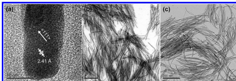
**Figure 4.** (a) High resolution and (b) normal TEM images of 12 nm × 500 nm sized FeP nanowires and (c) normal TEM images of 7 nm × 600 nm sized FeP nanowires.
