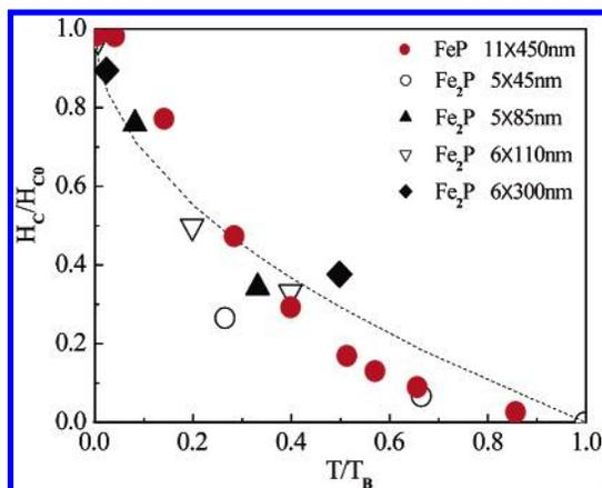
**Figure 10.** Normalized coercive field ( $H_c/H_{c0}$ ) is plotted for a normalized temperature ( $T/T_B$ ) for five different FeP and Fe<sub>2</sub>P samples, where  $H_{c0}$  is an estimated coercive field at  $T = 0$  K and  $T_B$  is the measured blocking temperature of each sample. The line is for the theoretical curve for a single domain of fine particles (see the text).
